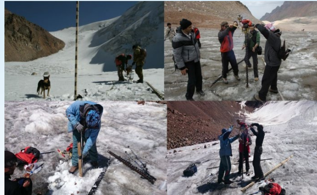
Drilling stakes into the glacier
