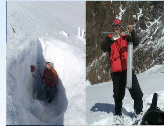
Snow density measurements
